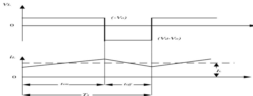
Fig. 2 Triggering Pattern for Boost Converter Pulses
