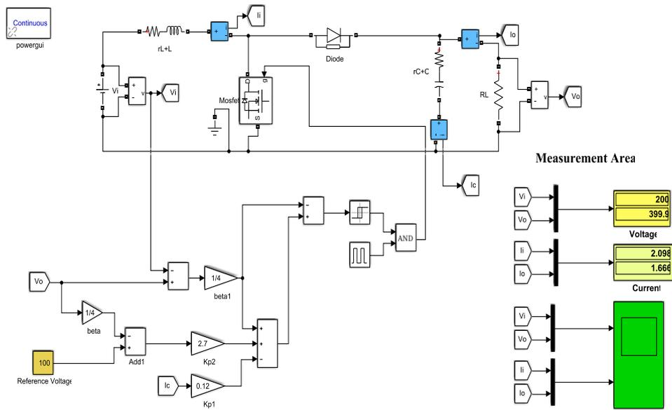
Fig. 5 Slide mode control of Boost Converter at 200 V to 400 V
