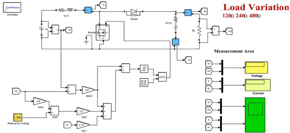
**Fig. 11** Slide mode control of Boost Converter value of Load
