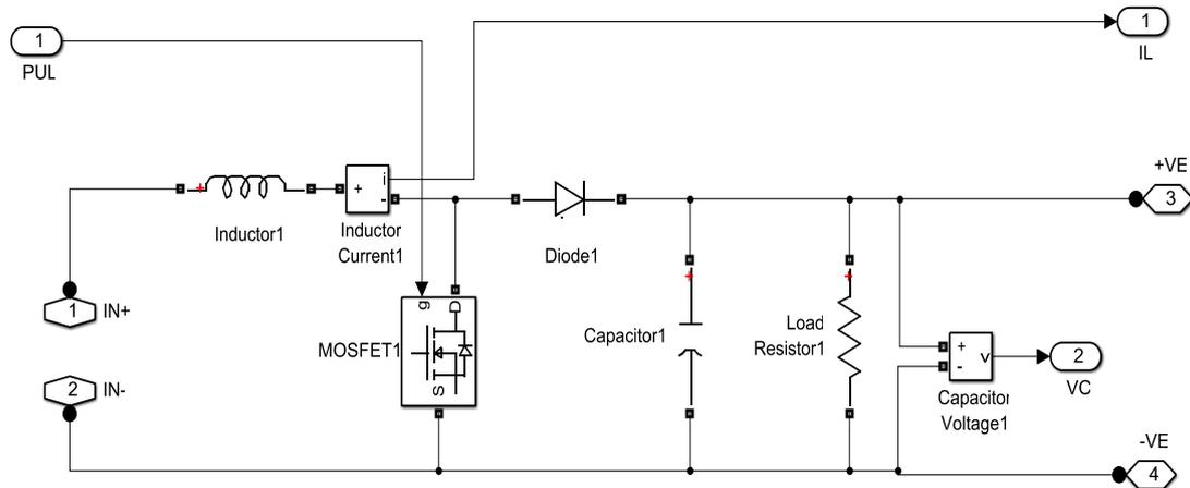
Fig.4 MATLAB model for Boost Converter
