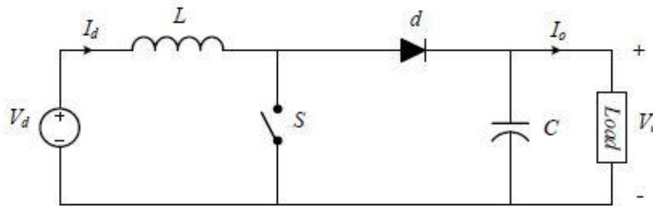
Fig. 1 Equivalent Circuit of Boost Converter
