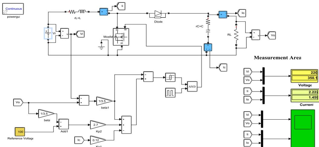
**Fig. 8** Slide mode control of Boost Converter at 220 to 350 V
