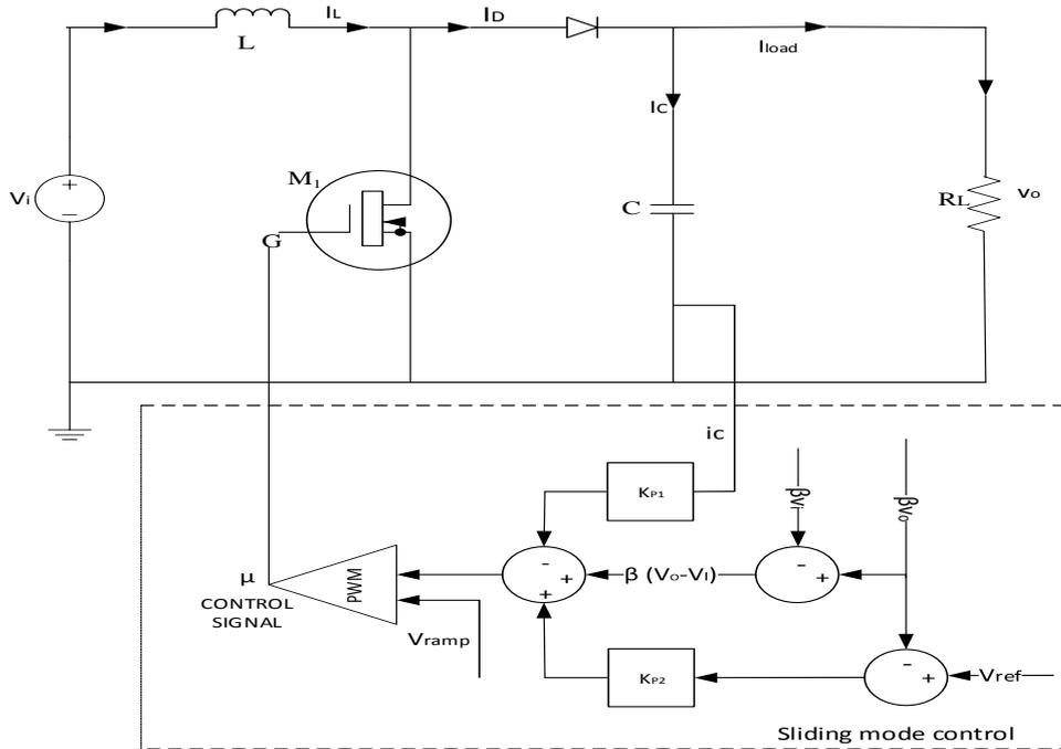
Fig. 3 Boost Converter describing Sliding Mode Control Law
