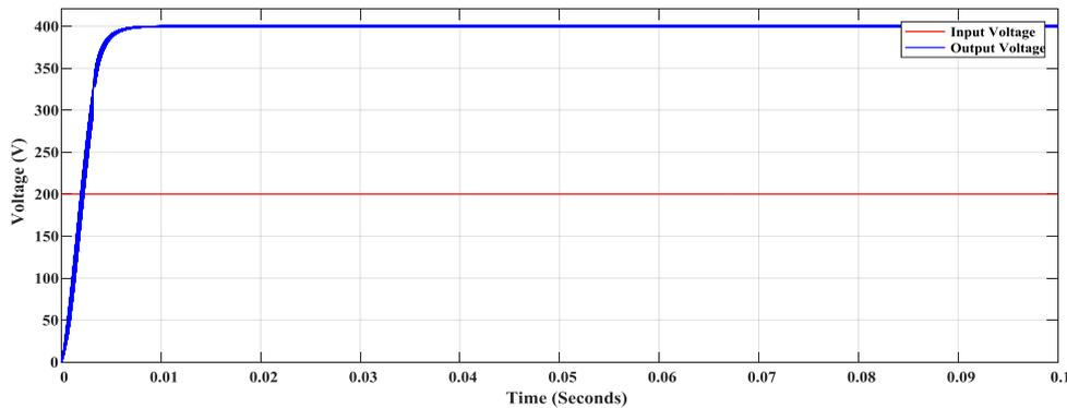
Fig. 6 Comparative analysis of Voltage Waveform for Boost Converter at 200 V to 400 V modes.
