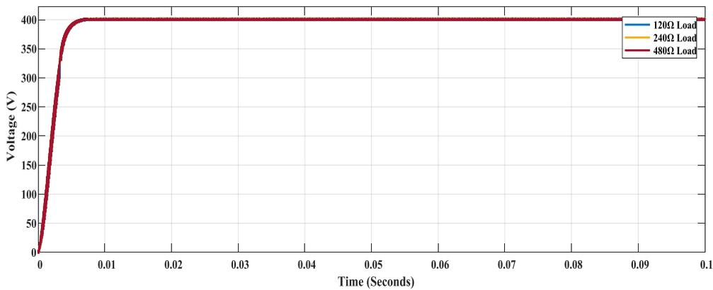
**Fig. 12** Output Voltage from Boost converter operating at different load resistance.
