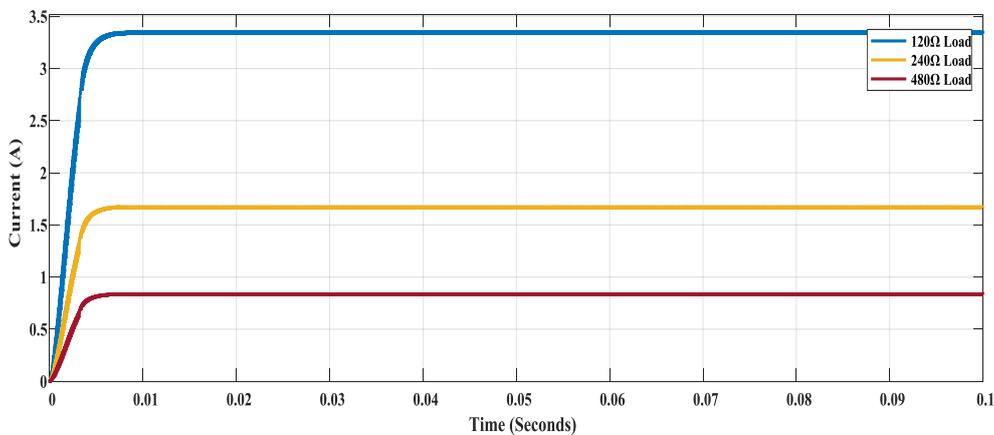
**Fig. 13** Output Current from Boost converter operating at different load resistance
