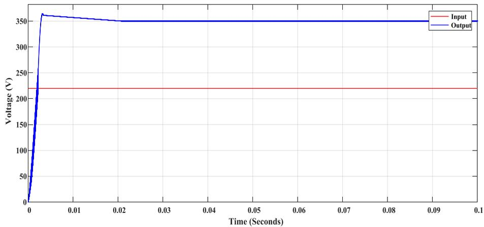
**Fig. 9** Comparative analysis of Voltage Waveform for Boost Converter at 220 V to 350 V mode
